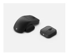
Three components that work together. The mouse core, tail extension, and thumb support create a traditional mouse that's light and portable. Or use by itself for a compact mouse.
